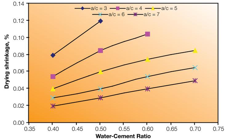
**FIGURE 3.** Effect of Aggregate-Cement Ratio (a/c) and Water-Cement Ratio on Drying Shrinkage [8]. (Data from 5 in. (125 mm) square mortar and concrete specimens exposed to a 70 °F (21 °C), 50 percent relative humidity environment for six months.)
